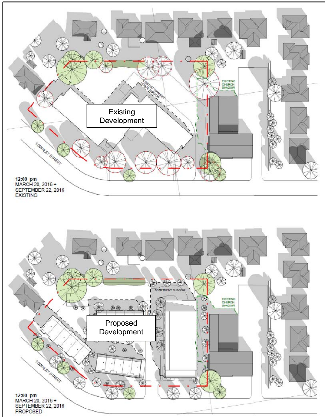
Figure 10: Shadow Study of Existing and Proposed Development at Noon during Equinox (Provided by HCMA Architecture and Design)
